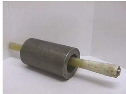
Fig.C.1 - 10. Anchoring of the bar in the chuck
