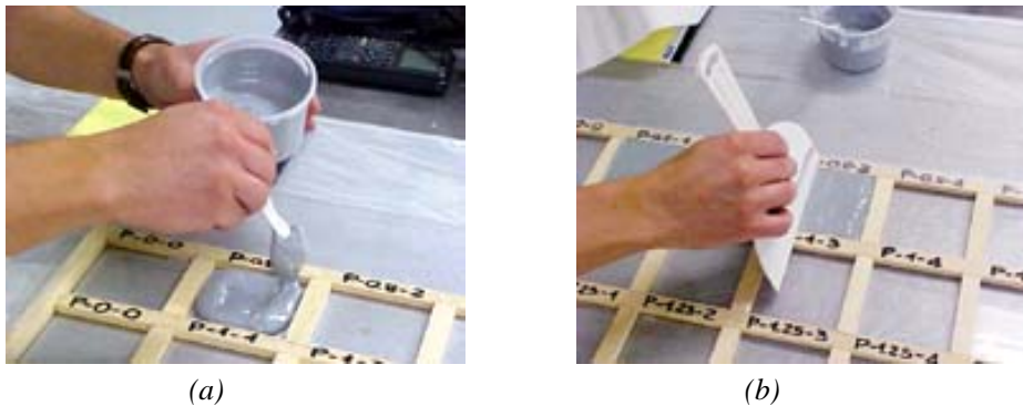
Fig. 4.47. Preparation of the specimens
