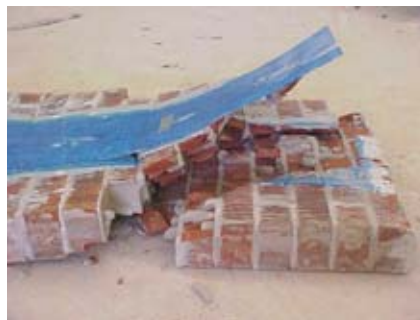
(b) BG9 – Shear failure
