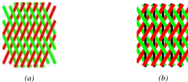
Fig. 2.8. Biaxial and triaxial braided fabric
