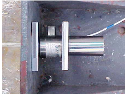
(b) Detail of the pressure transducer
