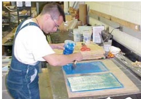
Fig. 4.12. Final impregnation of laminate plies
