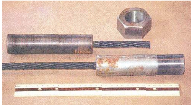
Fig. 7.7. CFCC tendon and anchor components
