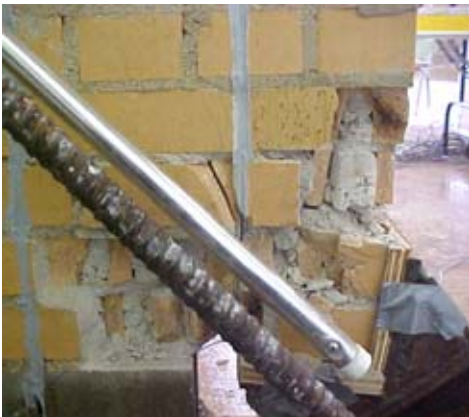
(a) Wall CLW5 after being tested (front)
