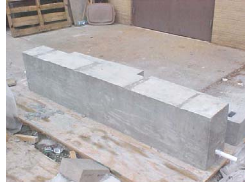
(b) RC beam after curing
