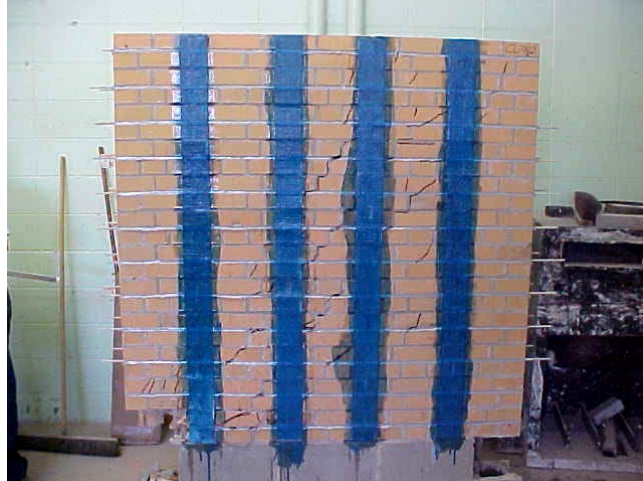
Fig.B.3 - 10. Wall CLW3 after failure (front)
