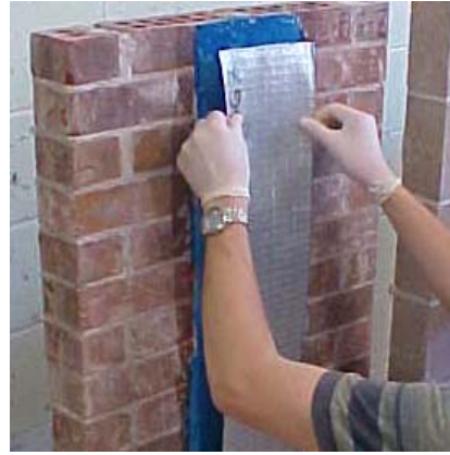
(a) (b) Fig. 3.5. FRP sheets and placement of the sheet
