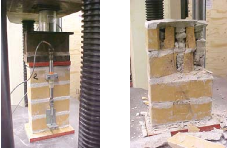
Fig. 4.6. Light clay prism before (a) and after failure (b)
