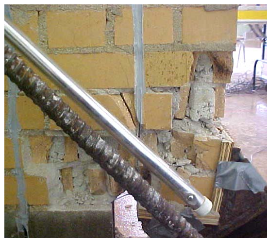
(b) Crushing of the corner (back)
