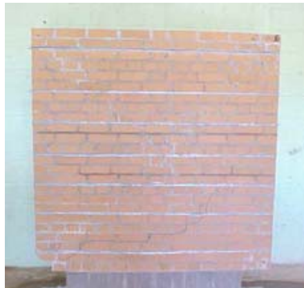
(b) Crushing of the corner (back)
