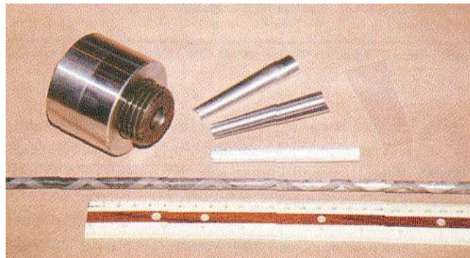
Fig. 7.5. Leadline tendon and anchor components
