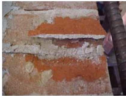
(f) Control B – Crushing of the midspan
