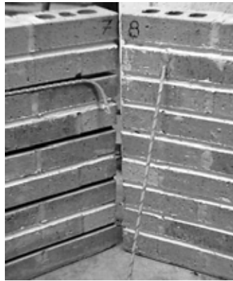
Fig. 6.4. GFRP rods in mortar bed joints (Tinazzi, 2000)
