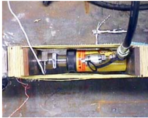
Fig. 4.28. Detail of hydraulic jack and pressure transducer
