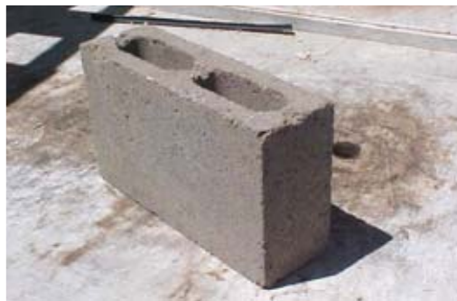
Fig. 4.1. Concrete block unit
