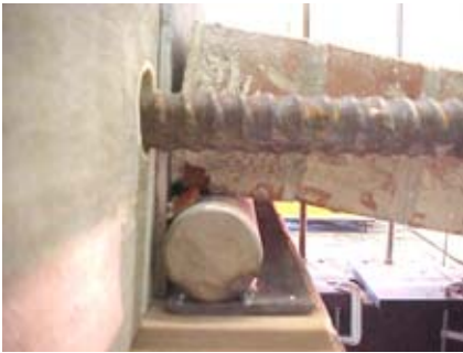
(a) BG5 – Crushing of the tile
