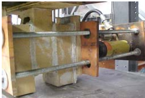
Fig. 4.9. Clay triplet under loading
