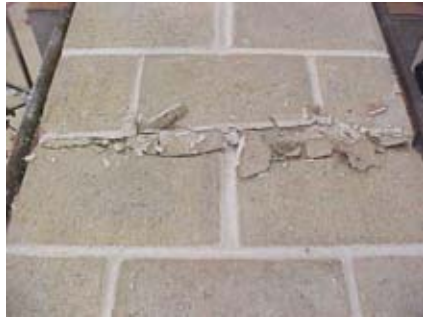
(c) Control C – Crushing of the midspan
