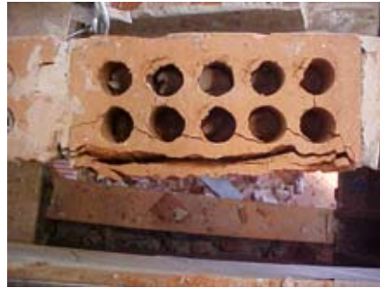
(b) BG3 – Crushing of the tile
