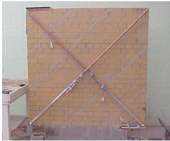
Fig.B.3 - 22. Wall CLW6 after failure (front)
