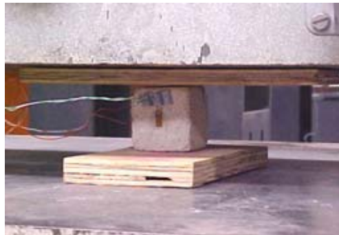
Fig. 4.10. Mortar cube under loading
