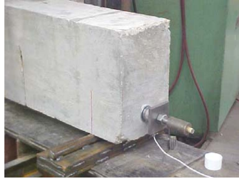
(b) Dead end and pressure transducer
