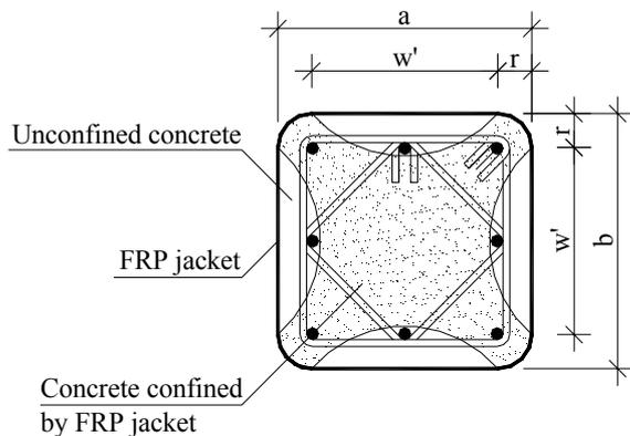
Figure 2. Strengthening effect in column with rectangular cross-section
