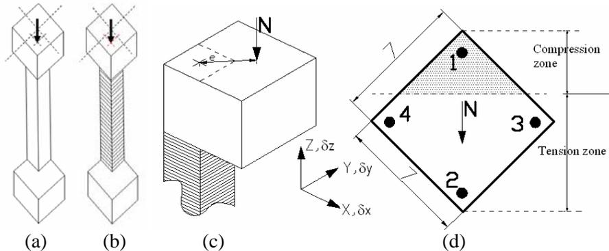
Figure 1. (a) column geometry, (b) Confined column, (c) Application of the load, (d) column cross section
