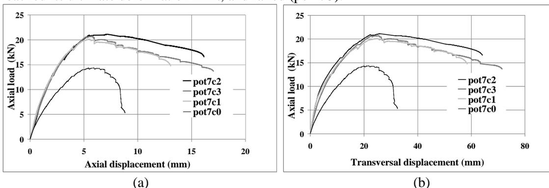
Figure 3. Load according to (a) axial displacement  $\delta z$  (b) transversal displacement curves  $\delta t$ . In the case of the confined columns the phenomenon of damage is different; in Fig. 3 the slope of this branch is quasi constant, compared to the unconfined column, the load decreases slowly
