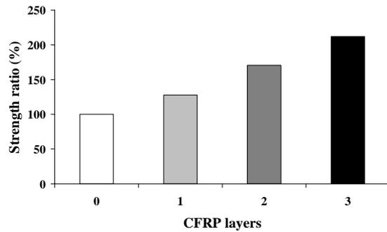
Figure 5. 10x10x20cm axially loaded strength columns according to CFRP layers number
