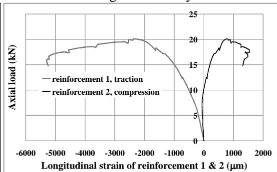
Figure 7. Load according to tension and compression steel reinforcements
