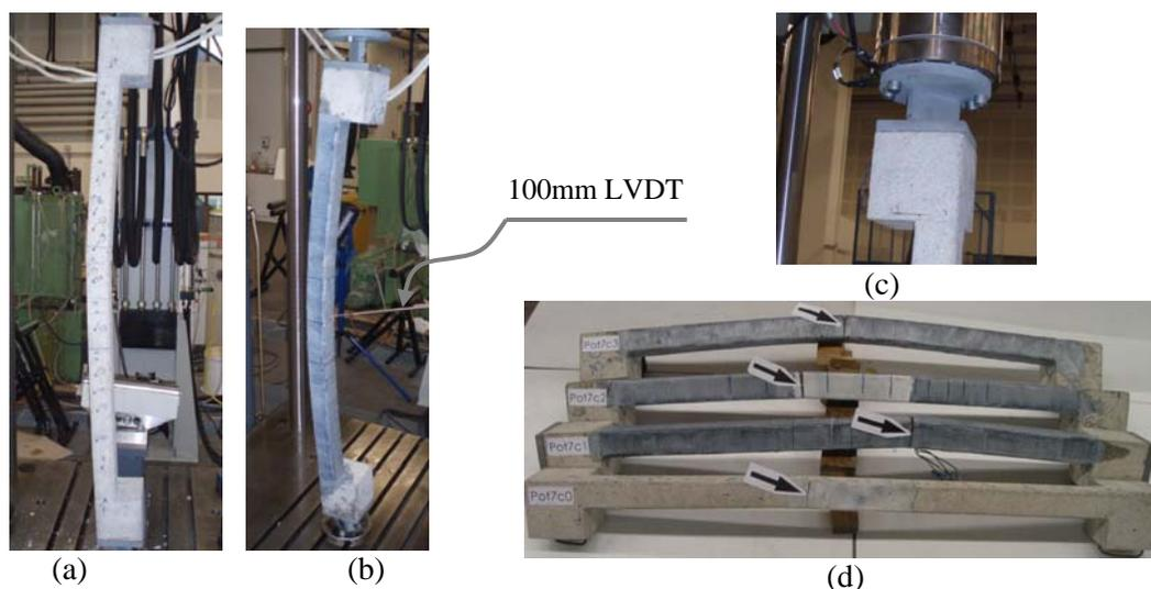
Figure 3. (a) Unconfined column buckling, (b) Confined column buckling, (c) Top mechanism of loading, (d) Columns major crack positions after test (at the arrowhead).
